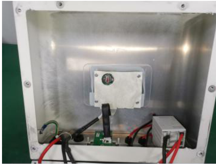
PIC3: Sample Photo, after IP6X test, no dust inside
