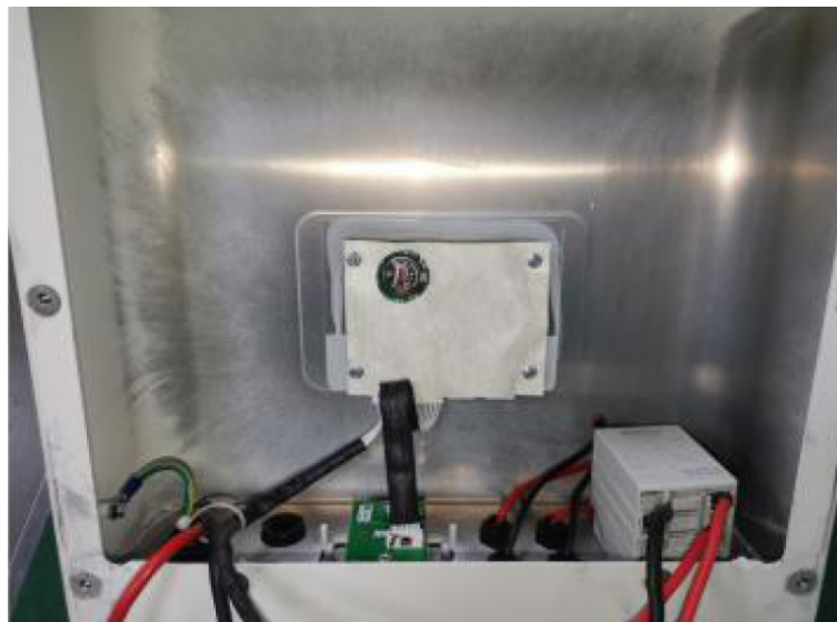
PIC6: Sample Photo, after IPX5 test, no water inside
