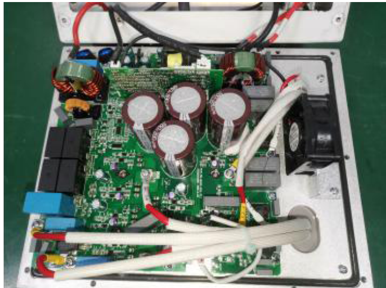
PIC2: Sample Photo, after IP6X test, no dust inside
