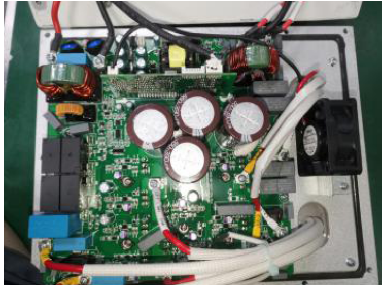
PIC5: Sample Photo, after IPX5 test, no water inside
